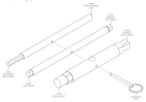
Slide unused corresponding tool through center hole of desired tool and secure with locking pin. See image below for reference.
